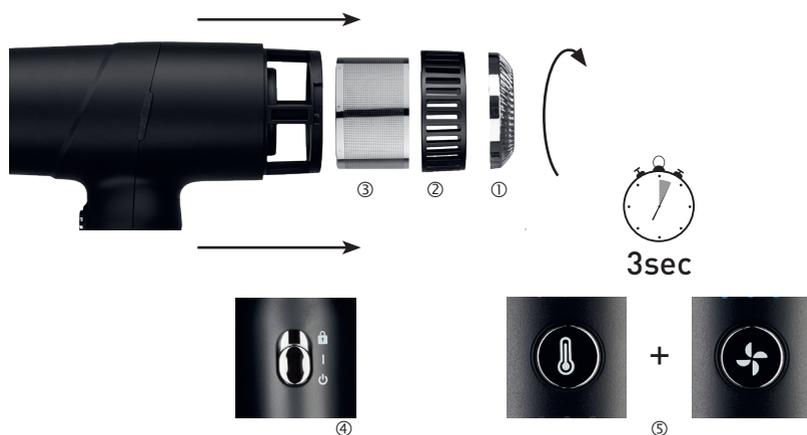
To activate the self-cleaning function, switch the device to the „⏻“ (standby) position. ④
